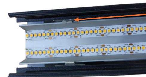
Figure 4: Internal tray with LED strips mounted to the housing
